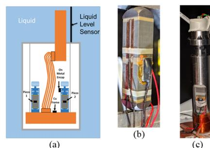
Figure 1: (a) Schematic view of the inside of the can, (b) Ceramic stack with Cernox sensor attached, (c) Picture of encapsulated piezo with geophone on top.
