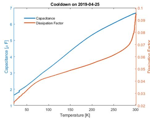
Figure 3: Dependency of the capacitance and dissipation factor of the PICMA™ piezo-stack versus temperature.
