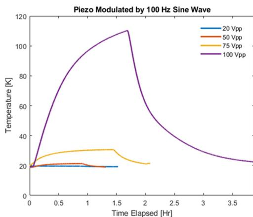
Figure 6: Piezo warm-up (from  $T=20\text{K}$ ) versus amplitude of sinewave stimulus pulse ( $V_{pp}$ ). Frequency of the sinewave  $f=100\text{Hz}$ .
