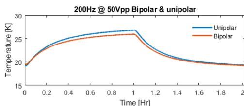
Figure 9: Piezo driven with sinewave stimulus pulses  $V_{pp}=50V$ : unipolar (0V to 50V) and bipolar (-25 V to 25 V).
