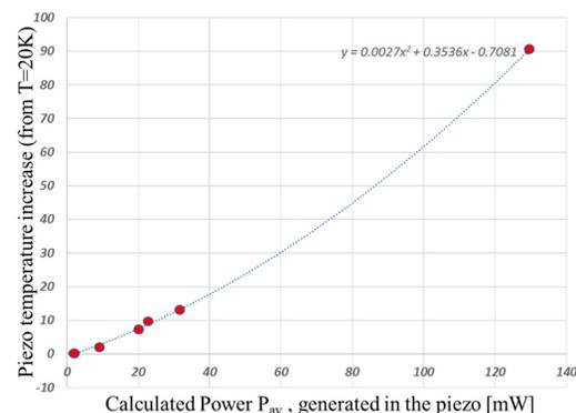
Figure 8: Piezo warm-up (temperature raised from  $T=20\text{ K}$ ) versus calculated power  $P_{av}$  (formula 1).
