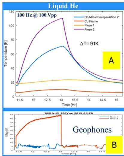
Figure 5: Test of the piezo warm-up, when piezo run with sinewave stimulus pulse with parameters:  $f=100\text{ Hz}$  and  $V_{pp}=100\text{ V}$ . (A) Temperature of all 4 RTD sensors inside enclosure, (B) Response of the geophone, mounted on the piezo.
