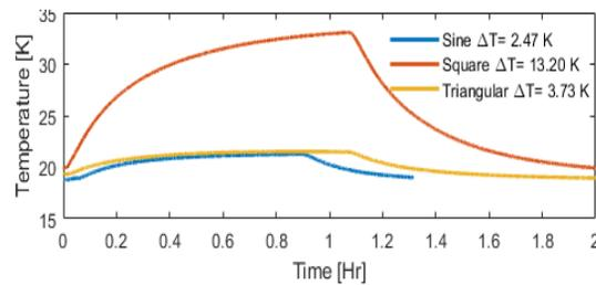
Figure 10: Piezo driven at  $f=100$  Hz and  $V_{pp}=50$  V with three different wave form: sine, square and triangular.
