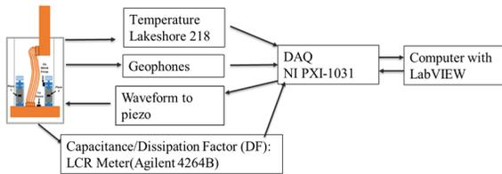
Figure 2: Schematic of data acquisition.
