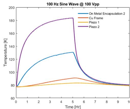
Figure 4: First test with liquid nitrogen. Piezo run with sinewave pulses with  $f=100$  Hz and amplitude  $100V_{pp}$ .
