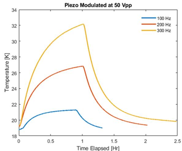
Figure 7: Piezo warm-up (from  $T=20\text{ K}$ ) versus frequency of sinewave stimulus pulse ( $f$ ). Amplitude of the sinewave  $V_{pp}=50\text{ V}$ .
