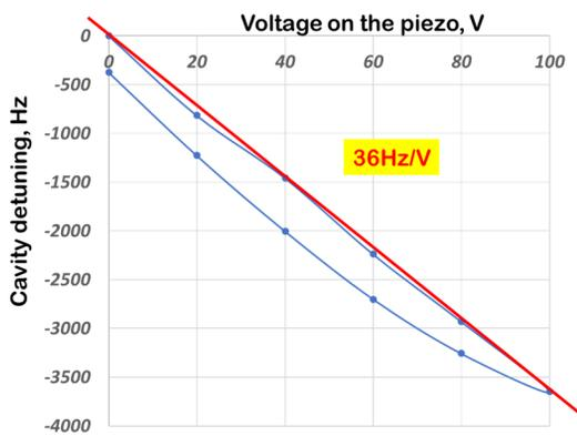
Figure 5: Cavity detuning with the piezo tuner.
