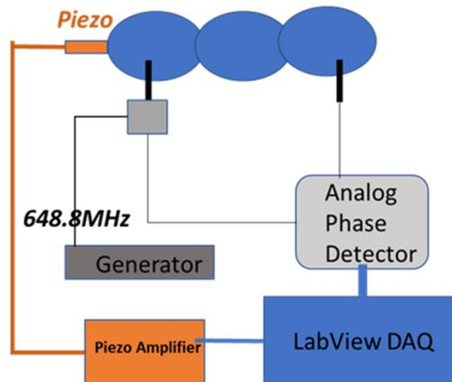
Figure 6: Setup to measure cavity transfer function.
