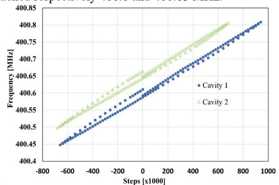
Figure 7: Tuner 300 kHz cycle at 2 K.
