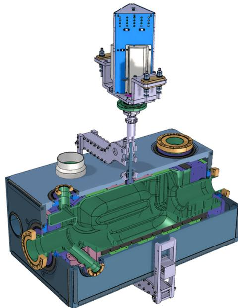
Figure 1: Cut-away view of the RFD tuner.
