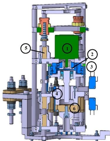
Figure 3: Cut-away view of the linear actuator.
