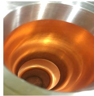
Figure 15: Chemical polished copper cavity substrate.
