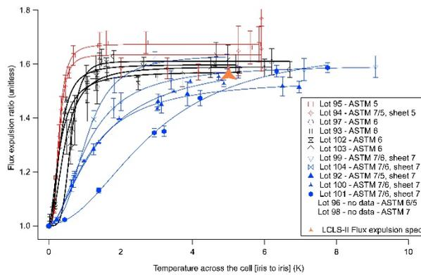
Figure 1: Flux expulsion vs. thermal difference (temperature across the cell) between iris's when the cells equator reached 9.25K. Each color represent each ASTM grain size defended by the manufactured lot, and the symbols are for each lot. Each curve is fit with a Hill-equation as a guide to the eye.
