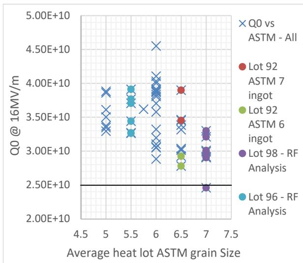
Figure 2: Q0 @ 16MV/m vs Average heat lot ASTM grain size. The light blue "x" is all data available, with other subsets of data overlapped in closed circles.
