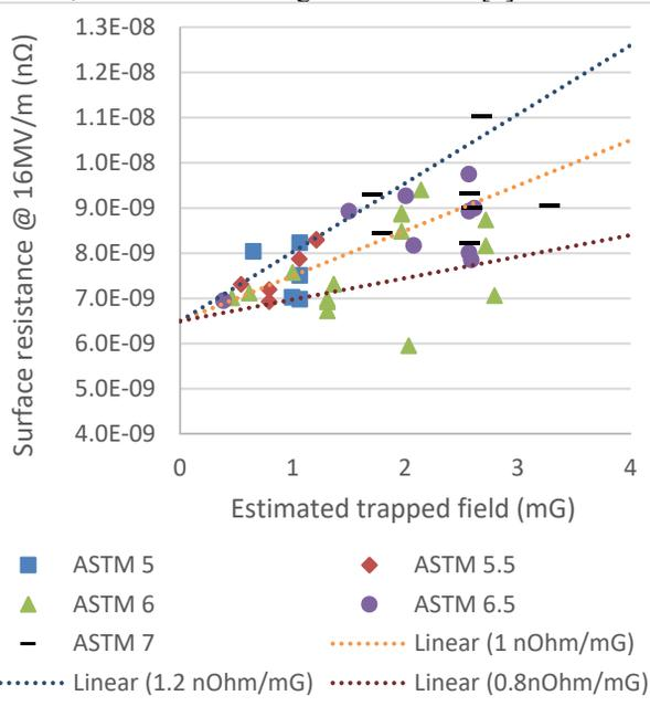
Figure 3: Estimated trapped magnetic field vs Q0 @ 16MV/m for the 43 9-cell cavities with magnetic field monitoring during cooldown. Each symbol represents a different average ASTM grain size. The three linear curves are the trapped magnetic field losses for 2N6 doping (centroid and error).
