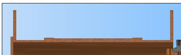
Figure 4: Cross section of the mandrel of the superconducting solenoid, featuring GA-optimized steps for improving field uniformity.
