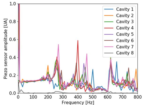
Figure 16: Piezo response to a longitudinal load.
