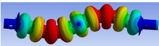
Figure 10: Example of a cavity mode (152Hz).
