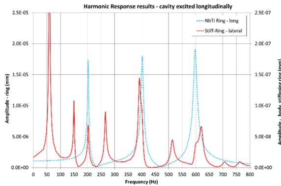
Figure 11: Cavity response to a longitudinal load.
