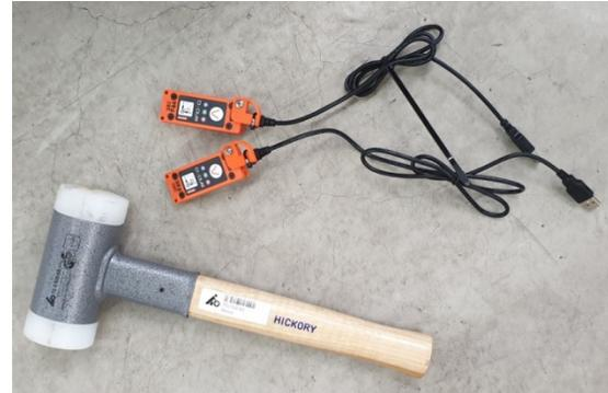
Figure 13: “Hammering test” tools.
