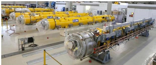
Figure 1: EXFEL cryomodules at DESY Hamburg.
