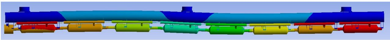
Figure 8: The first mode of the cold mass with string.
