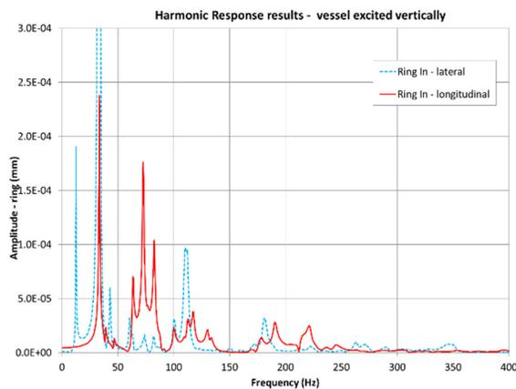
Figure 12: Vessel frequency response to a vertical load.
