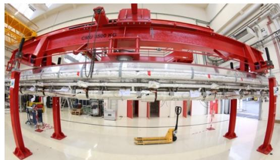
Figure 3: EXFEL cold mass with string at CEA Saclay.
