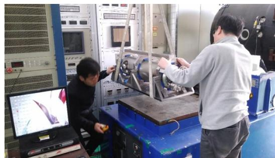
Figure 8: Vibration Test Setup.
