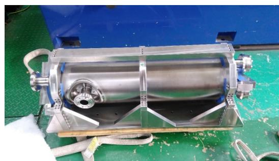
Figure 9: Fixture for QWR Cavity for Vibration Test.
