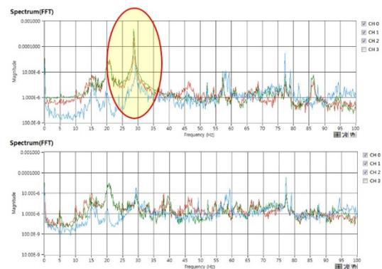
Figure 2: Disturbance from Cold-Box (upper – turn-on, lower – turn-off).
