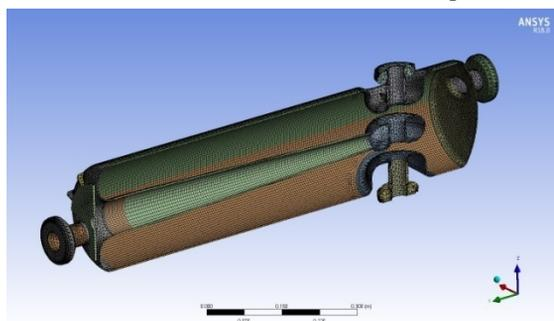
Figure 4: Modelling of unjacketed QWR SC Cavity.
