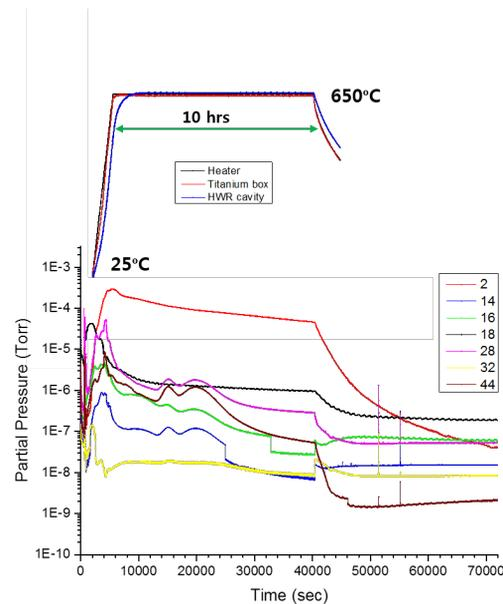
Figure 3: Temperature profile during the heat treatment (top) and RGA analysis (bottom): The maximum partial pressure peak of hydrogen (red line),  $3 \times 10^{-4}$  Torr, appears at around 2 hours.
