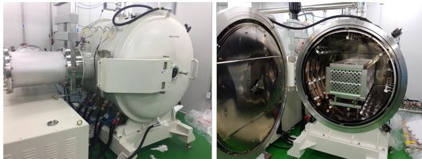
Figure 1: Vacuum furnace for the heat treatment in the SRF cleanroom: Cavity is loaded horizontally in the furnace with titanium box.
