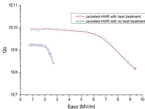
Figure 5: Quality factor ( $Q$ ) vs. acceleration electric field gradient ( $E_{acc}$ ) of the jacketed HWR cavity at 2K: A red reversed triangle line and a blue triangle line represents the heat treated HWR and no heat-treated HWR, respectively.
