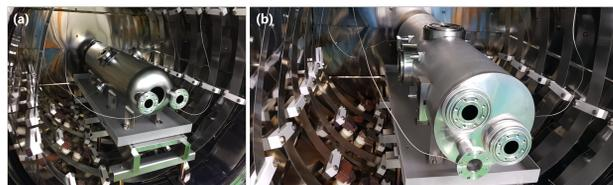
Figure 2: Horizontal loading of the jacketed and bare HWR cavity in the vacuum furnace: (a) bare HWR cavity and (b) jacketed HWR cavity.
