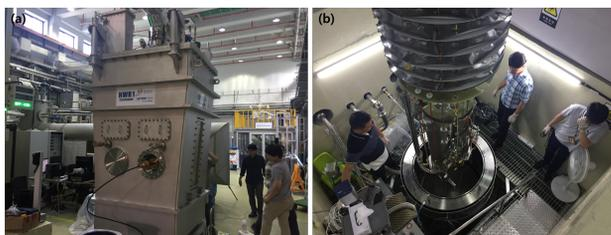
Figure 4: Cavity test: (a) cryomodule test in which the jacketed cavity is integrated with RF power coupler and tuner and (b) vertical pit test, in which bare or jacketed cavity is inserted with only variable coupler.
