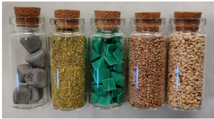
Figure 2: Applicable abrasive: SiC, Diamond, Al 2 O 3 , coconut, corn.
