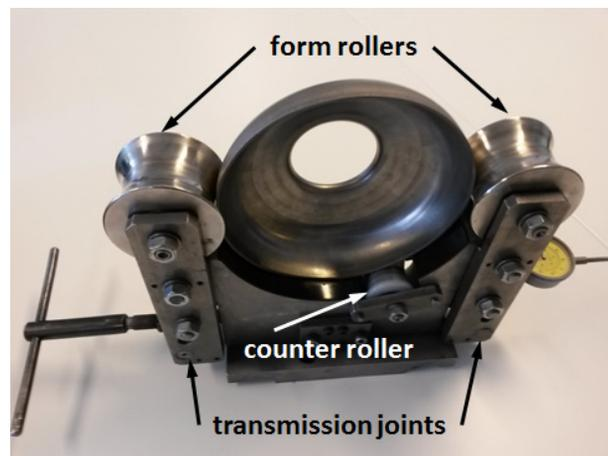
Figure 4: Rolling device with cavity half-cell.
