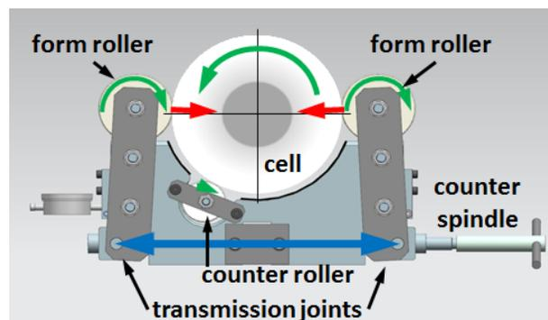
Figure 5: Principle of rolling device.
