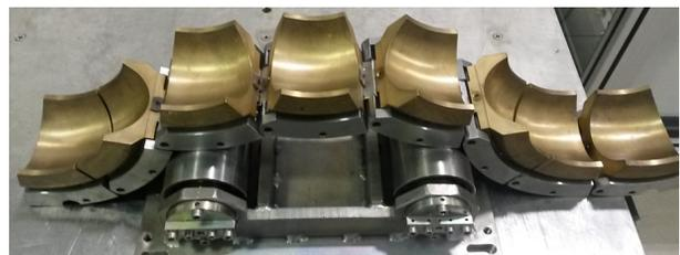
Figure 1: Opened stainless steel tuning chain with eight brass pressing shoes.
