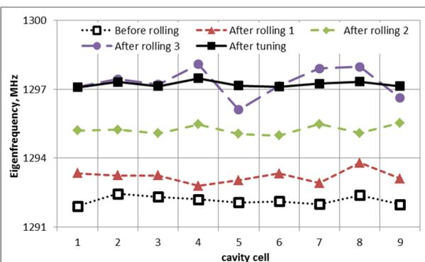
Figure 7: Cavity cells eigenfrequencies before and after each of 3 rolling.
