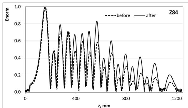
Figure 8: Normalized field distribution  $|E(r=0,z)|$  on cavity axis for second monopole mode TM011 – before rolling (dash line) and after final standard tuning (solid line).
