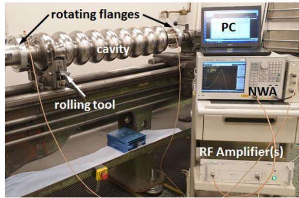
Figure 6: Radial tuning with rolling device and frequency control measurements.
