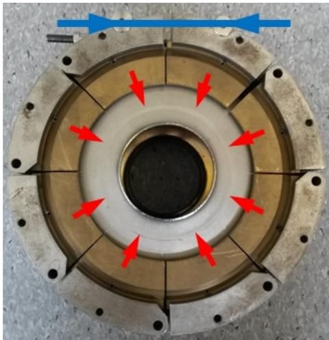
Figure 2: Closed tuning chain with cavity cell.
