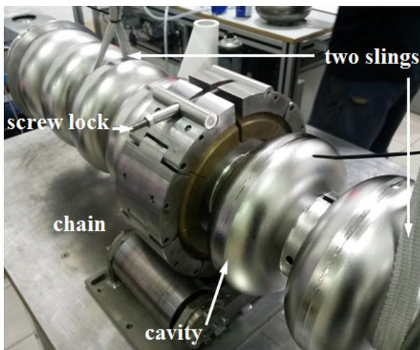
Figure 3: Tuning chain installed to cavity.
