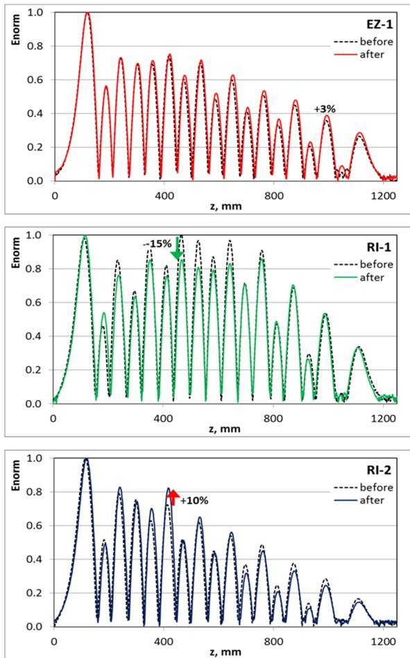
Figure 3: Normalized field distribution  $|E(r=0,z)|$  on cavity axis for second monopole mode TM011.
