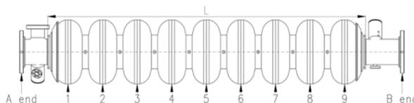
Figure 1: 9 cell cavity length ( $L$ ).
