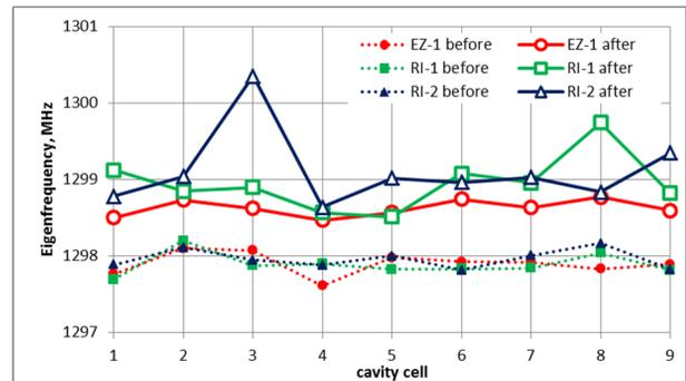
Figure 2: Eigenfrequencies of cavity cells before and after radial tuning.
