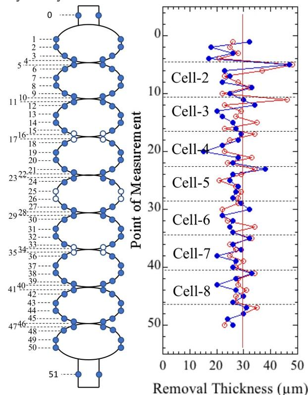
Figure 3: Removal thickness along the cavity length in VEP performed with cathode rotation at 50 rpm and unoptimized acid flow. The vertical line on the plots shows average removal thickness. The schematic in the left shows the positions where the removal thicknesses were measured.
