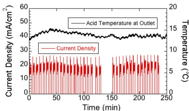
Figure 2: Cavity current density and acid temperature profiles during the VEP performed with cathode rotation at 50 rpm and unoptimized acid flow. The temperature was measured at the outlet of the cavity.
