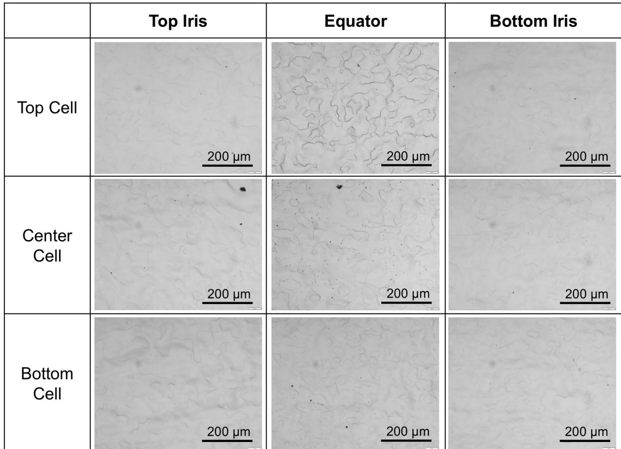
Figure 4: Optical microscope images of the nine coupons after VEP with cathode rotation at 50 rpm and unoptimized acid flow rates.
