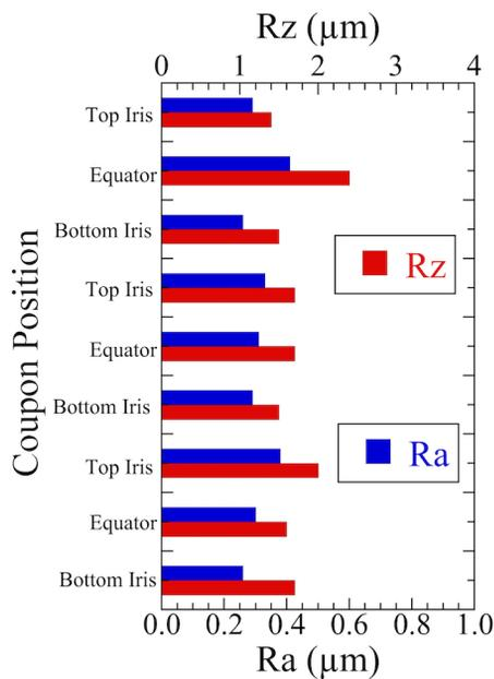
Figure 5: Coupon surface roughness Ra and Rz after VEP performed for an average removal of 30 μm at cathode rotation of 50 rpm and unoptimized flow rates.
