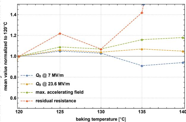
Figure 7: Normalised values of all studied parameters plotted over bake temperature.
