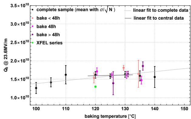
Figure 5: Quality factor measured at an accelerating field of 23.6 MV/m versus bake temperature.
