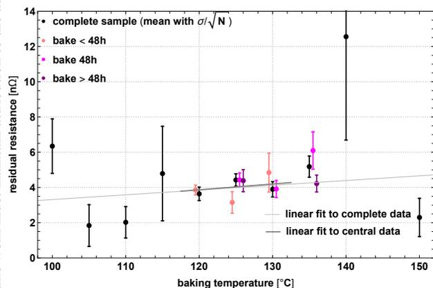
Figure 6: Residual resistance displayed over bake temperature.
