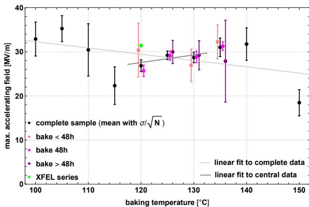
Figure 3: Maximal accelerating gradient displayed over bake temperature.
