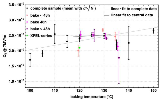
Figure 4: Quality factor measured at an accelerating field of 7 MV/m versus bake temperature.
