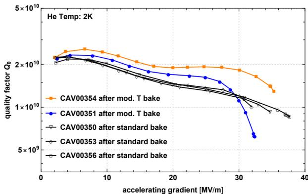
Figure 9:  $Q_0(E)$  for cavities which underwent the modified low temperature procedure, compared to their sister cavities which were treated with the standard procedure.
