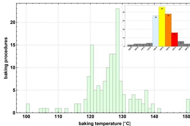
Figure 1: Temperature distribution of all cavity bake procedures. On the upper right, the binning, used in the analysis, is displayed.
