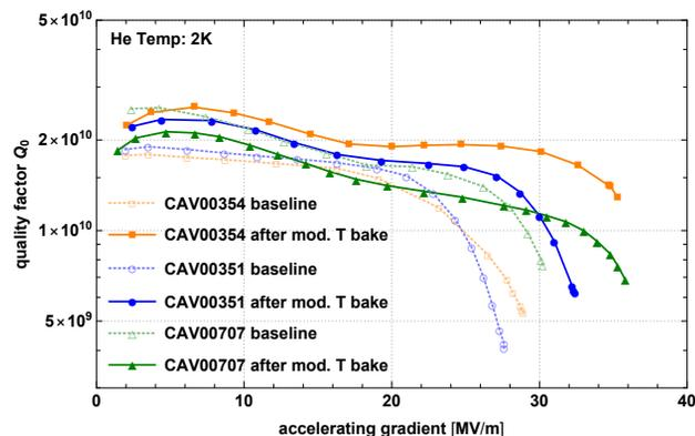
Figure 8:  $Q_0(E)$  curves for all cavities baked at DESY applying the modified low temperature procedure.
