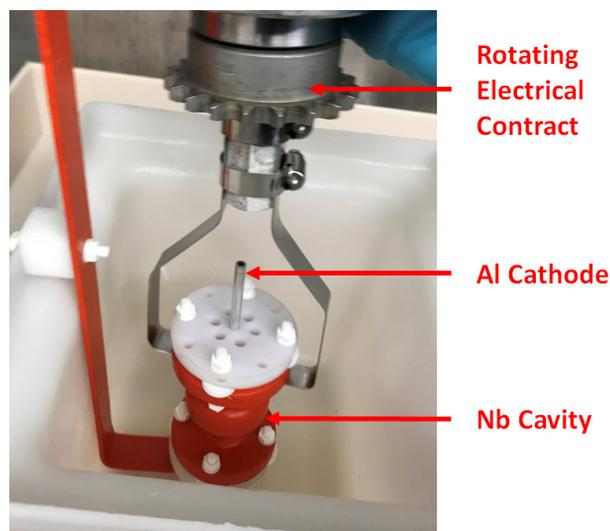
Figure 6: 5 GHz single-cell cavity EP.
