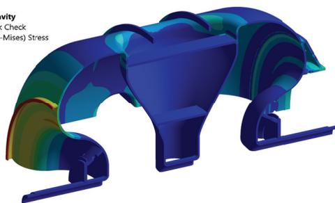
Figure 10: Equivalent VM stress during leak check.
