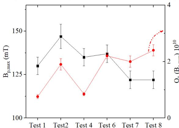
Figure 5: Summary of rf test results at 2.0 K.
