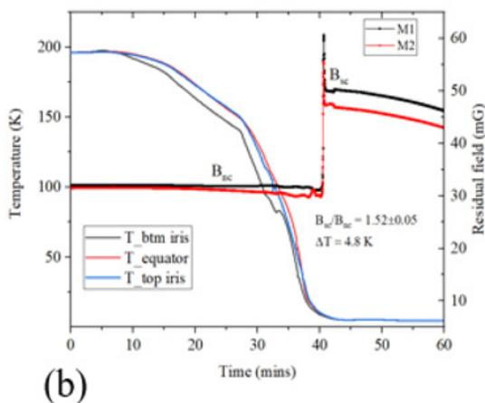
Figure 1: (a) Complete Meissner effect during cooldown showing the schematic of a single-cell cavity with flux-gate magnetometers (M1, M2) and Cernox sensors (T1,...T6) and (b) Temperature and magnetic field during transition from normal to superconducting state measured during a cooldown cycle of the cavity.
