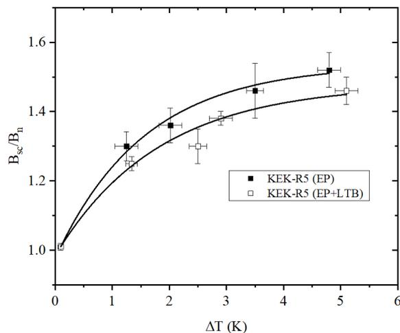
Figure 2: Flux expulsion ratio as a function of spatial temperature difference (iris-to-iris) for the cavity after EP and LBT. Solid lines are fits with a sigmoidal curve.
