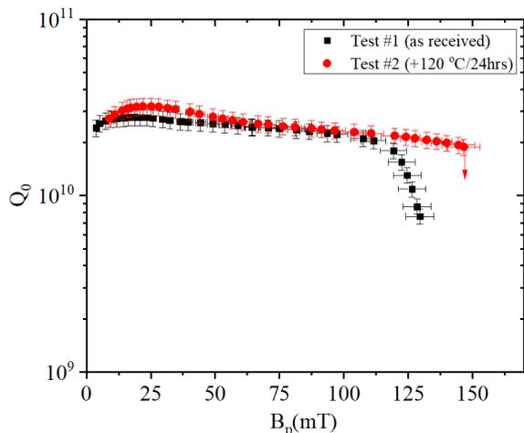
Figure 4:  $Q_0(B_p)$  at 2.0 K measured of the cavity in the as-received state and after LTB at 120°C for 24 hours. The cavity in the as-received state was limited by a  $Q$ -slope, whereas the cavity was limited by a quench after LTB.
