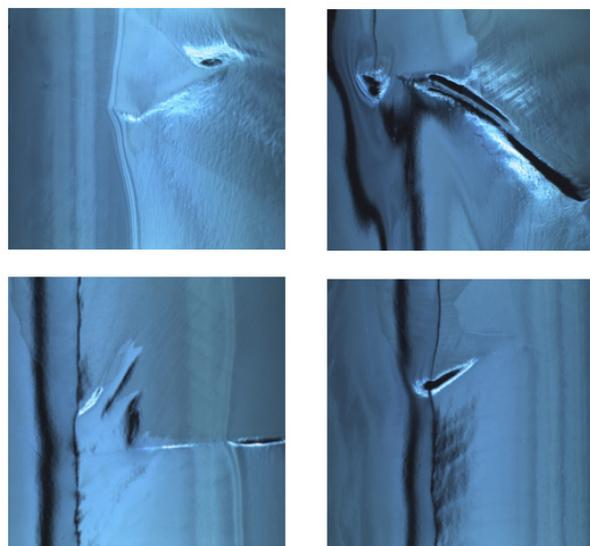
Figure 6: Optical photographs on the inner cavity surface near the equator.
