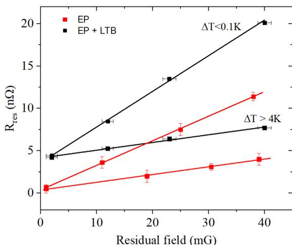
Figure 3: Residual resistance as a function of applied dc magnetic field measured for  $\Delta T < 0.1$  K and  $\Delta T > 4.0$  K after EP and followed by LTB, respectively.
