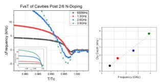
Figure 9: (Left) Frequency vs temperature data for cavities of different resonant frequencies subject to 2/6 N-doping. The lower left inset gives a zoomed-out picture of the FvsT profiles. (Right) Comparison of the dip depth versus the resonant frequency.
