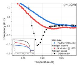
Figure 8: Frequency vs temperature data for a 1.3 GHz single cell cavity subject to three different surface treatments. The inset shows a zoomed-out plot of the three profiles.
