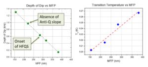
Figure 11: Effect of MFP on (Left) dip depth (Right) transition temperature.
