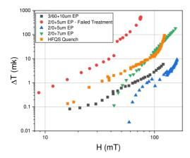
Figure 6: A log vs log plot of the measured temperature difference as a function of the peak magnetic field of the RTD located closest to the position of quench for each of the above TMAP studies. The He bath temperature was ~1.5 K. The heating profile of a cavity with high field Q-slope (HFQS) is shown in orange squares for comparison.
