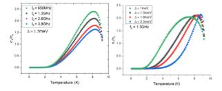
Figure 12: (Left) BCS calculations of the quasi-particle conductivity for various resonant frequencies of cavities with a superconducting gap of 1.5 meV. (Right) BCS calculations of the quasi-particle conductivity for various superconducting gaps for a resonant frequency of 1.3 GHz. Both figures are done for niobium with a T<sub>c</sub> of 9.25 K.
