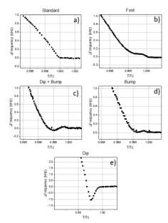
Figure 7: The five features observed in FNAL FvsT data. The normal conducting frequency is set to correspond to 0 Hz for each case.
