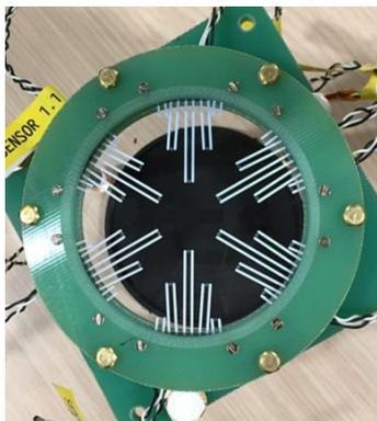
Figure 2: TES wafer used for cavity diagnostics.
