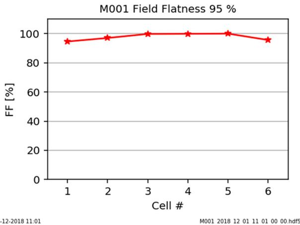
Figure 4: Field flatness of M001 after fabrication.
