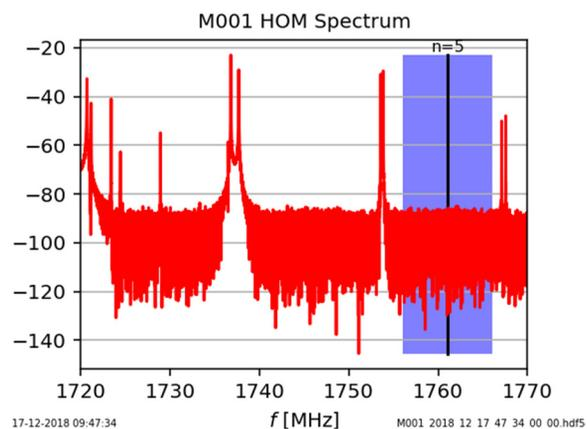
Figure 3: HOM spectrum at cold for M001, showing no mode within 5 MHz of the 5<sup>th</sup> beam harmonic.
