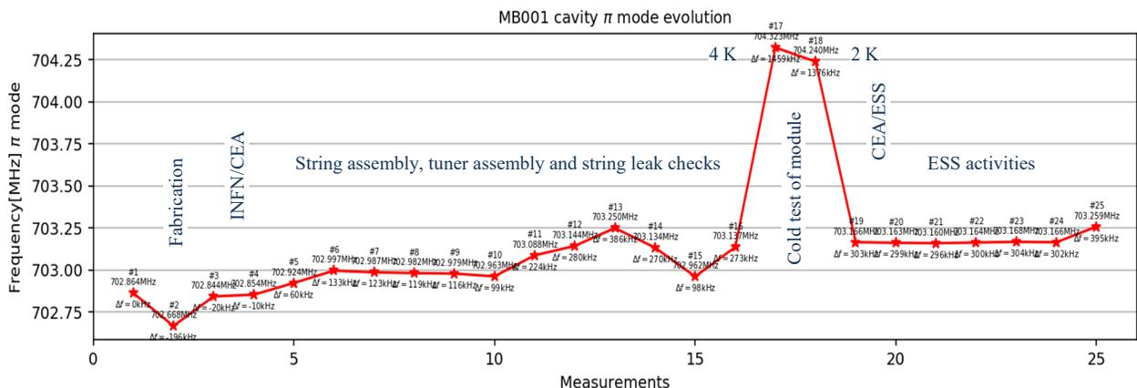
Figure 7: Frequency evolution of MB001 during cavity handover, module installation, test at CEA and handling at ESS.
