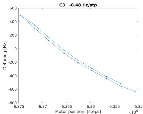
Figure 2: Frequency tuner scan for cavity 3 of XM50.1.
