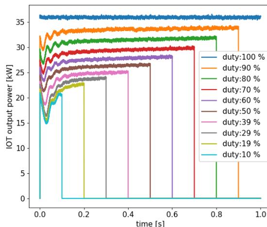
Figure 3: IOT amplitude transient as a function of duty cycle.
