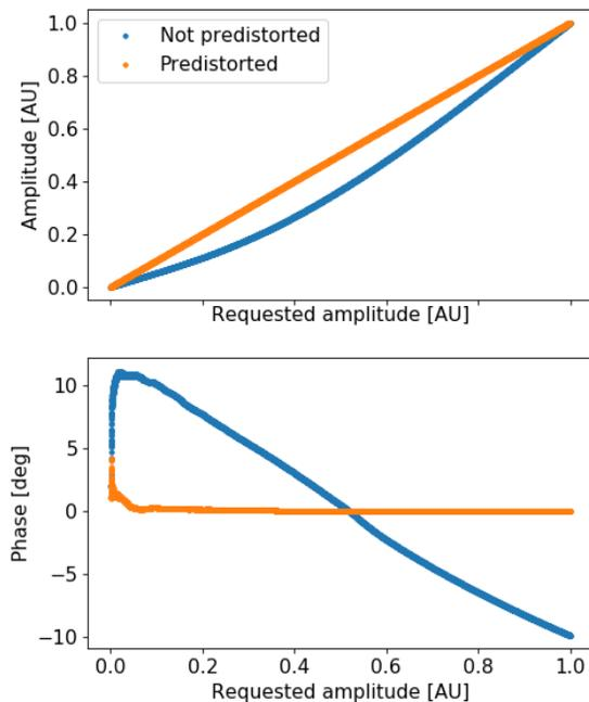
Figure 4: IOT amplitude (top) and phase (bottom) linearized using the pre-distortion module in the LLRF main controller firmware.
