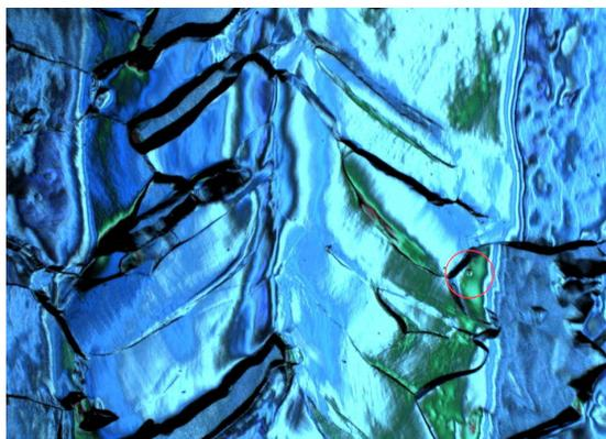
Figure 4: Picture with a cat's eye type defect in the vicinity of the EBW seam. The defect is marked by red circle.
