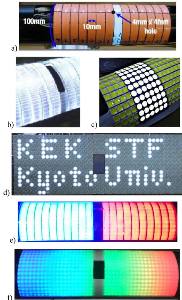
Figure 1: Changes of the illumination system. a) The first inorganic Electro-Luminescence (IEL) device (one strip lighted). b) Light emitting guide strip type using white LEDs. c) Armadillo type illumination with more LEDs (line by line). d) Pixel controlled Armadillo illumination. e) Blue and red stripes for refurbishment of old version. f) Colored pixel controlled Armadillo illumination. The camera holes are located at the centers.
