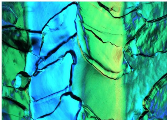
Figure 3: Picture taken with the color illumination. The color information has the slope of the surface.
