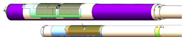
Figure 2: The modular design of the camera system allows adaptability to multiple cavity sizes. A larger cavity with working distance larger than an L-band cavity requires a larger lens system with larger diameter. It also allows easy maintenance by sending the short head part back to the manufacturer instead of the long cylinder.
