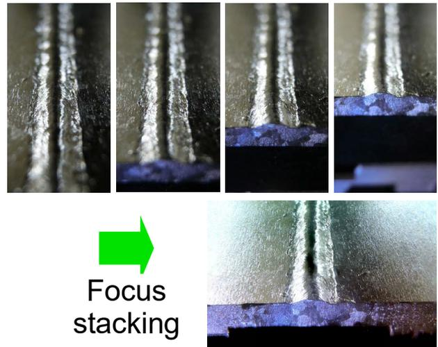
Figure 11: Focus stacking from pictures with different focus positions will eliminate the autofocus function.
