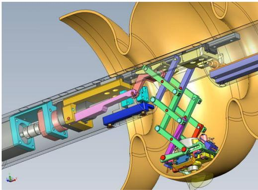
Figure 7: The original structure of the local grinding system, where the local grinding motor is located at the retractable grinding stage.
