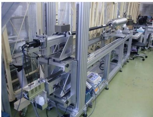
Figure 10: The combined Kyoto camera (top cylinder) and the local grinding system (bottom cylinder).
