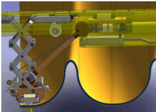
Figure 8: The improved structure of the local grinding system, where the local grinding motor is located at the end of the cylinder.
