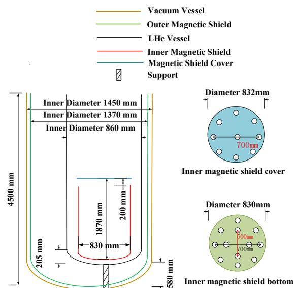
Figure 2: Vertical test dewar diagram.
