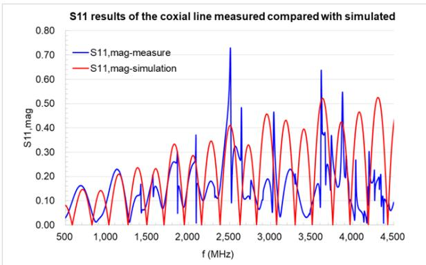
Figure 8: The reflection properties of the coaxial line prototype measured compared with simulated.
