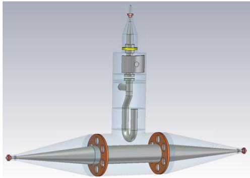
Figure 6: The coaxial transmission line with HOM coupler model.
