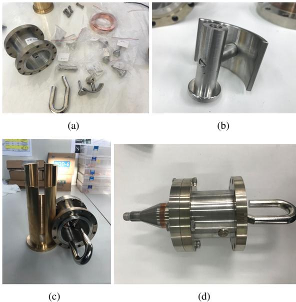
Figure 3: (a) Detachable parts, (b) T type inner conductor, (c) the fixture used for installation, (d) HOM coupler prototype.
