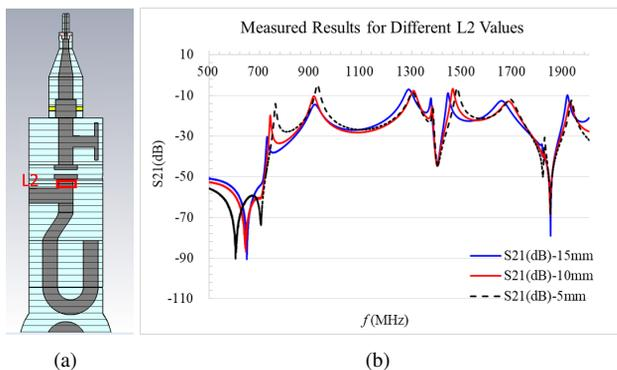
Figure 12: (a) HOM coupler model, (b) measured results for different L2 length.
