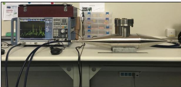
Figure 7: The coaxial transmission line prototype.
