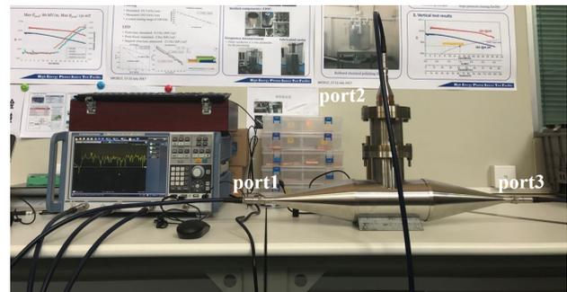
Figure 9: The coaxial transmission line test bench with HOM coupler.
