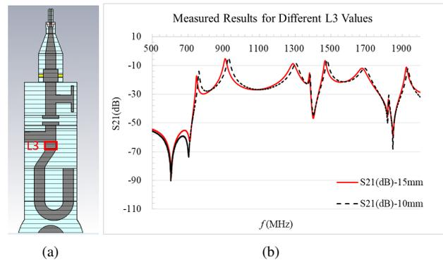
Figure 13: (a) HOM coupler model, (b) measured results for different L3 length.
