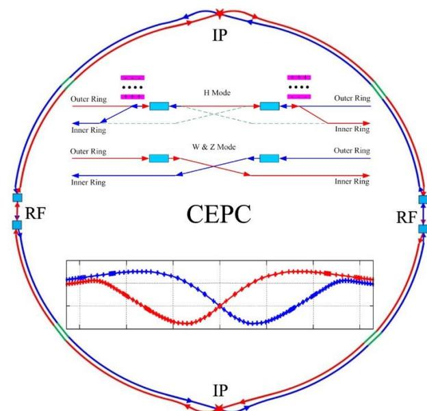
Figure 1: Layout of CEPC collider.
