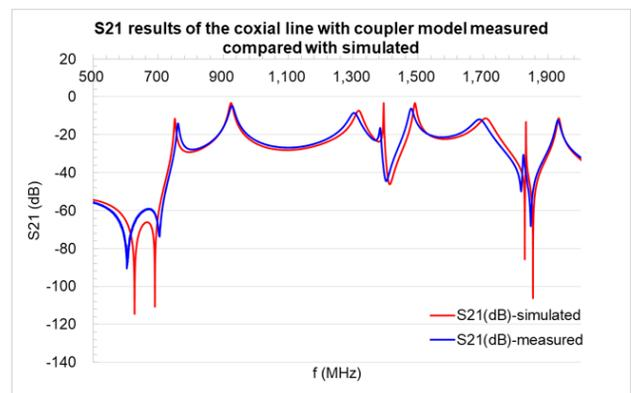
Figure 10: The measured S21 parameters of the HOM coupler compared with simulated.
