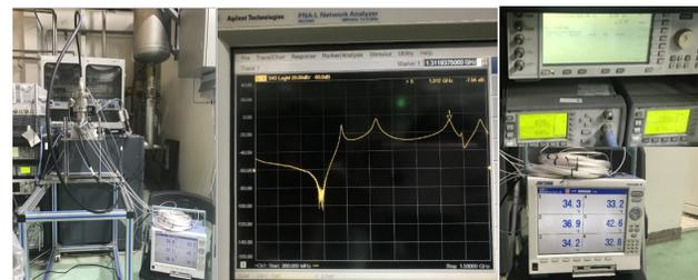
Figure 14: High power test for the HOM coupler at room temperature.
