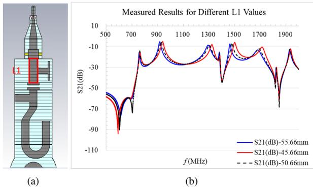
Figure 11: (a) HOM coupler model, (b) measured results for different L1 length.
