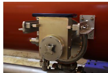
Figure 2: Photograph of waveguide to coaxial transition of the power coupler with adjustment knob for  $Q_{ext}$ .
