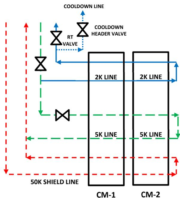
Figure 2: Cryogenic lines in the LERF.
