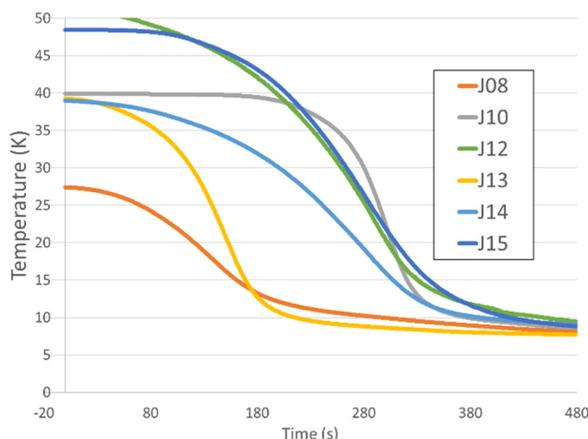
Figure 4: Cavity 1 cooling rates during FCD.
