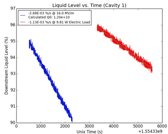
Figure 5: Q<sub>o</sub> Measurement: He Liquid level vs. electric heat and RF heat.
