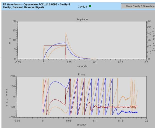
Figure 6: Cavity waveforms during QL and cavity probe Q measurements.
