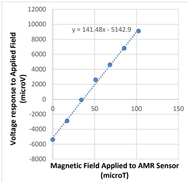
Figure 4: Sensitivity of AMR sensor at 77K.
