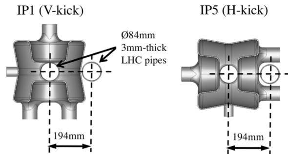
Figure 1: The DQW cavity satisfies the LHC geometric constraints imposed by the second beam pipe to provide a deflecting kick for both vertical and horizontal crossing planes.
