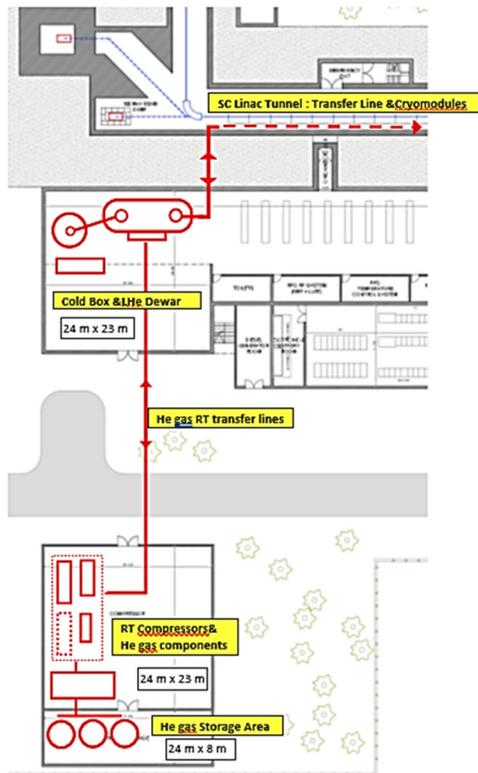
Figure 3: Schema for MINERVA Linac and cryogenic plant buildings.
