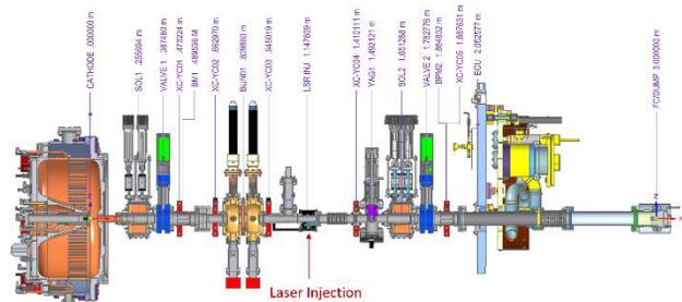
Figure 1: Injector source beamline.
