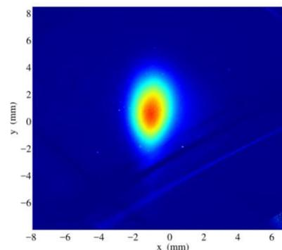
Figure 5: First photocurrent beam from the gun.
