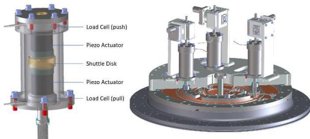
Figure 3: Details of the tuners used to push or pull the gun anode plate.
