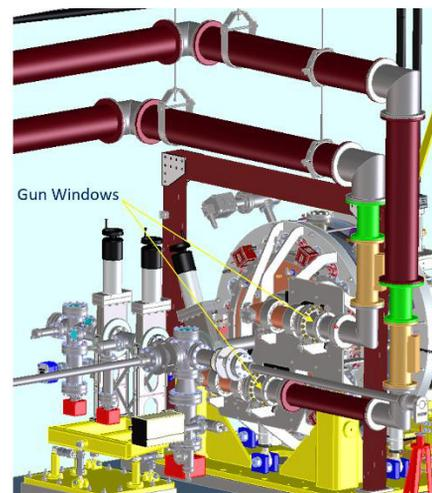
Figure 2: Layout upstream of the gun showing the waveguide connections and cathode load-lock system.
