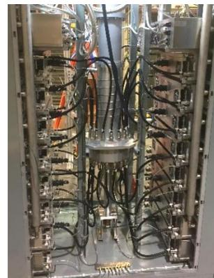
Figure 4: Photo of the inside of one of the 60 kW SSAs showing the 30-to-1 coaxial RF combiner.
