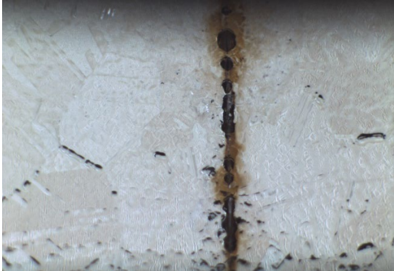
Figure 7: Representative image of seam weld cracks discovered in low surface field Cu cavities, LSFC-12 shown here, after SUBU acid etching.
