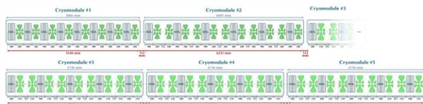
Figure 2: Layout of the 5-cryomodules SRF Linac.
