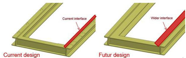
Figure 5: Widening of support frame interface for cavity string assembly.
