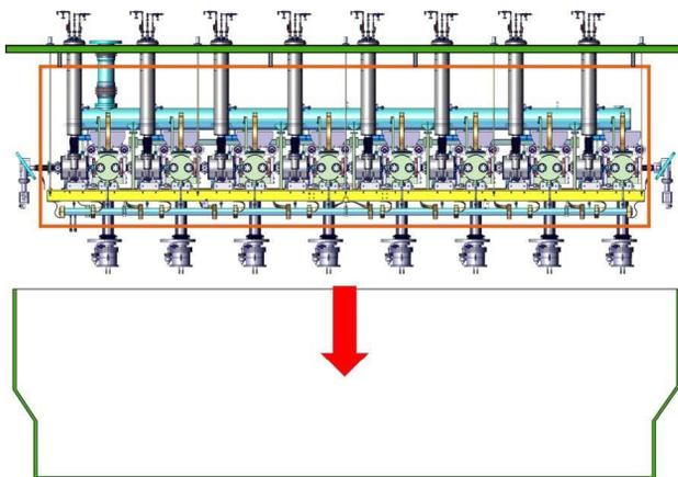
Figure 4: Conceptual design of the DONES cryomodule and principle of the insertion of the cold mass (upper mock-up) in the vacuum vessel (lower sketch).
