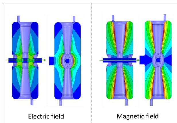
Figure 3: Field distribution in the high beta cavity.
