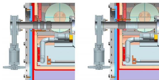
Figure 10: Beam pipe end assembly. On the left: the previous design. On the right: the new design.
