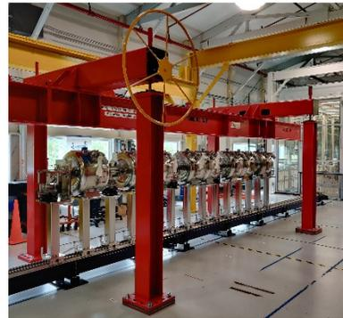
Figure 6: String assembly under the lifting tooling.
