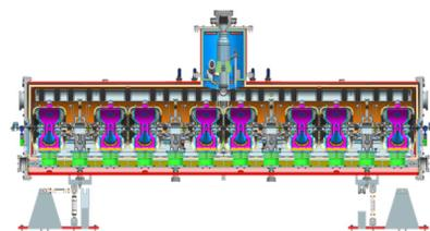
Figure 2: SSR1 cryomodule configuration.
