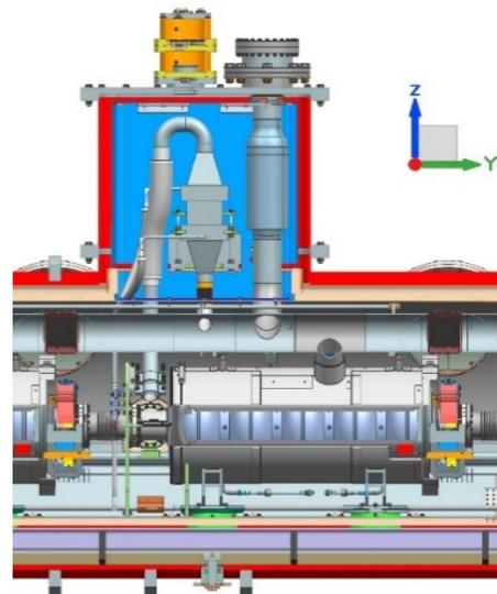
Figure 9: Interface with the relief line and heat-exchanger.
