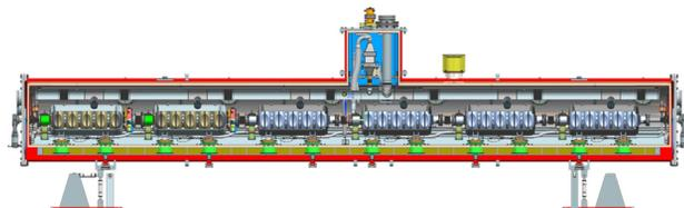
Figure 3: HB650 cryomodule configuration.
