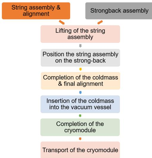
Figure 4: Assembly sequence of SSR1, SSR2, LB650 and HB650 cryomodules.
