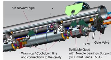
Figure 2: Solid model of cold mass.
