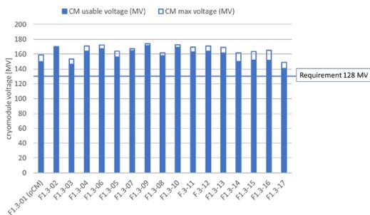
Figure 3: Cryomodule Voltage Gain.
