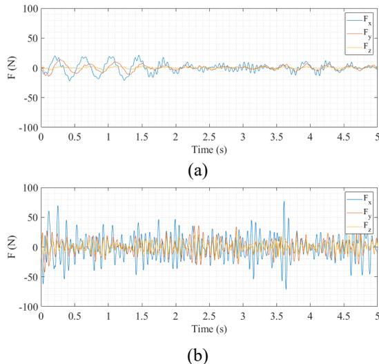
Figure 10: Force on a reference bellows – a) TT equipped with helical isolators; b) rigid TT.
