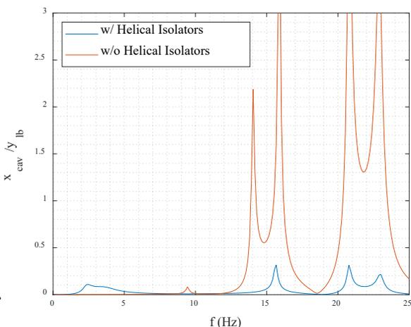
Figure 8: FRF of the vertical displacement of the reference cavity – With and without helical isolators.
