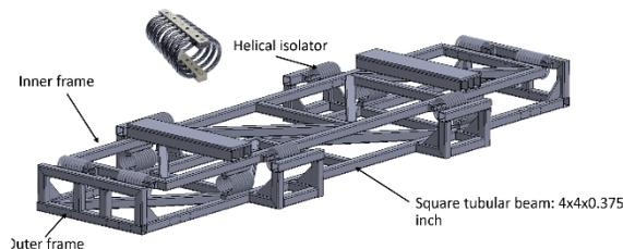
Figure 7: Drawing of the TT with helical isolators.
