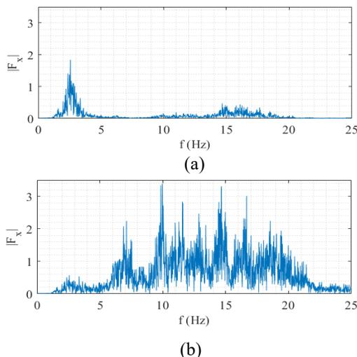
Figure 11:  $x$ -component of the force on a reference bellows. a) TT equipped with helical isolators; b) rigid TT.
