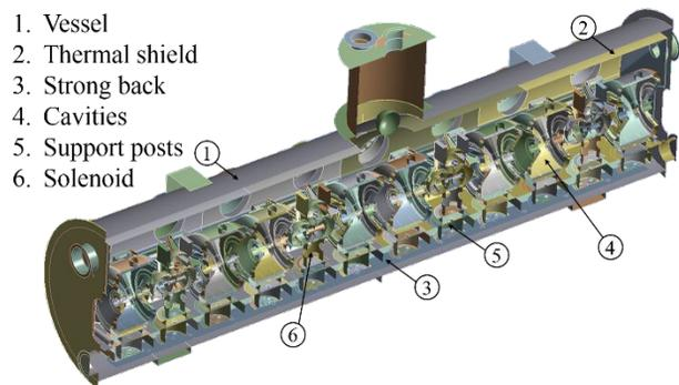
Figure 1: Main subassembly of the FE model.
