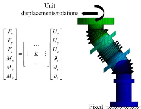
Figure 3: Equivalent stiffness matrix computation.
