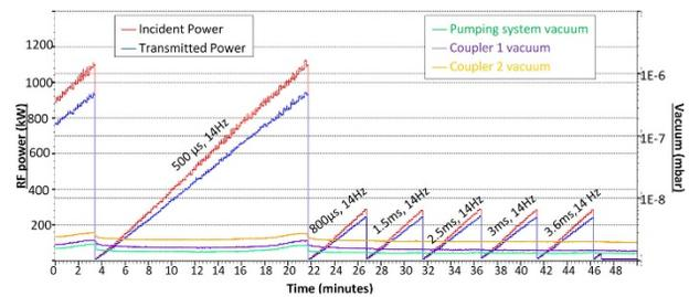
Figure 16: Standing wave 14 Hz (1<sup>st</sup> position of the short circuit).
