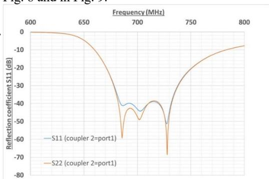
Figure 8: Reflection coefficient.
