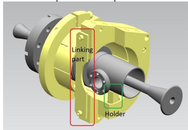
Figure 10: The 5K thermal interface (yellow) with the linking part and the holder.
