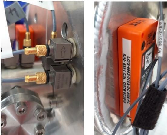
Figure 8: The coupler with the sensors.
