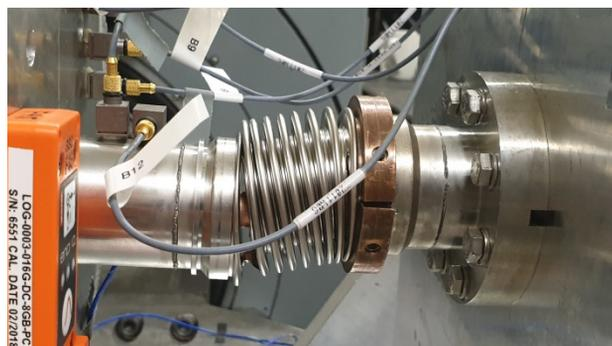
Figure 13: The bellows after the failure at test 3.
