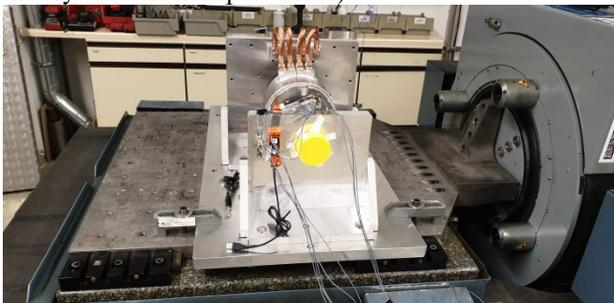
Figure 9: The coupler on the shaking table.
