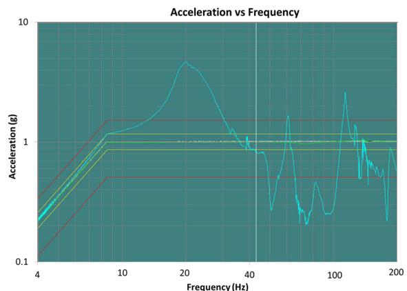
Figure 11: Acceleration vs frequency at the coupler port during the first sweep test (test 1).
