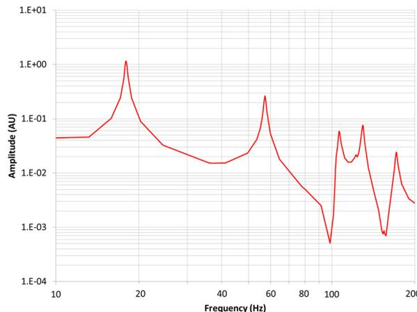
Figure 6: The harmonic response at the 80 K interface.
