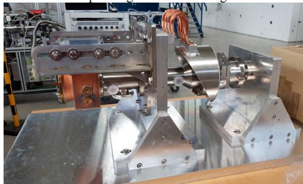
Figure 7: The coupler on the test support.
