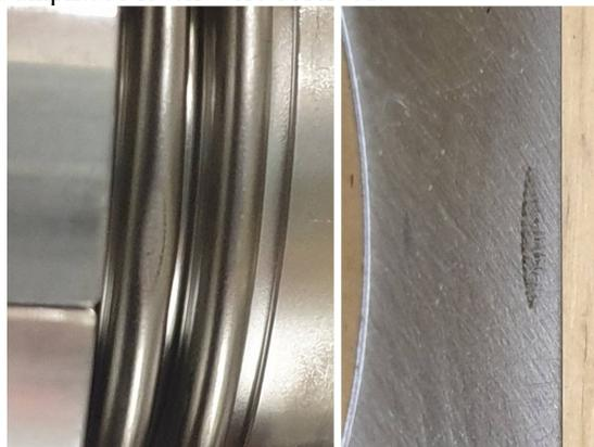
Figure 12: Left, the dent on the bellows – right, the damage on the linking part.
