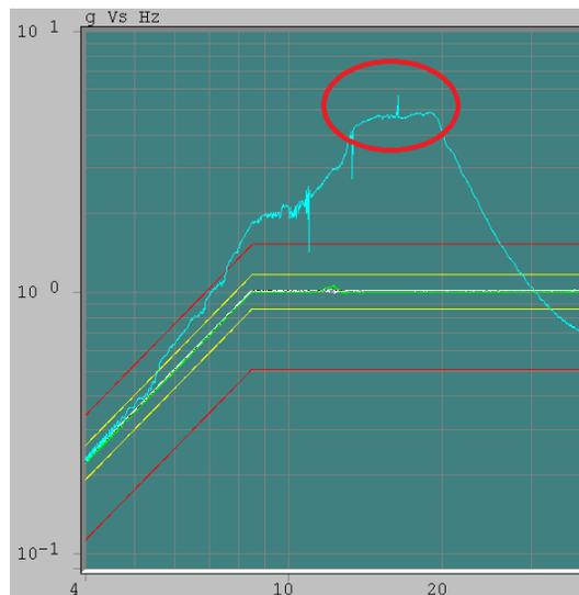
Figure 14: The acceleration vs frequency profile during the bellows failure.
