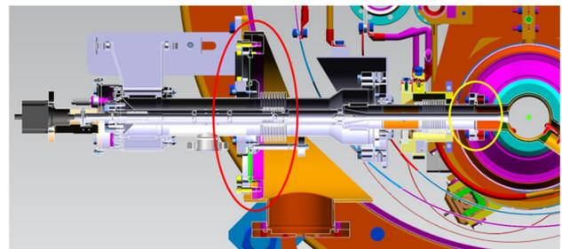
Figure 2: Section of an EXFEL coupler assembled in the cryomodule; in red and yellow the connections to the module (fixed points).
