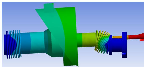
Figure 5: The profile of the 1st Eigenmode.
