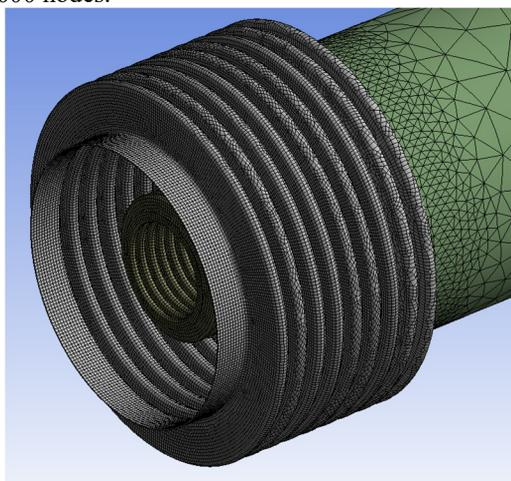
Figure 4: A detail of the mesh.
