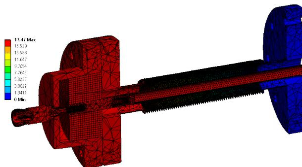
Figure 3: Test coupler deformation under 1 kN.
