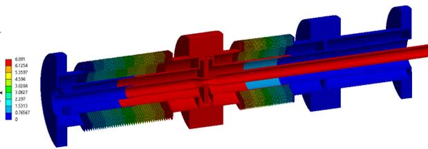
Figure 8: Power coupler deformation under 3 kN.
