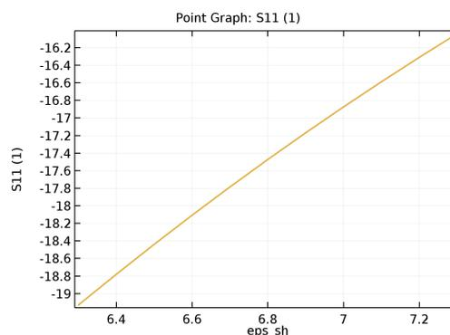
Figure 2: Test coupler reflection over ceramics dielectric coefficient.
