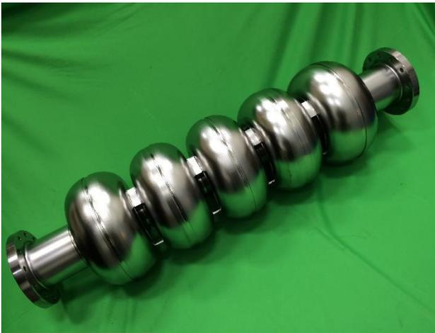
Figure 2: 5-cell LSF shape cavity LSF5-1 as completed electron beam weldment at JLAB.
