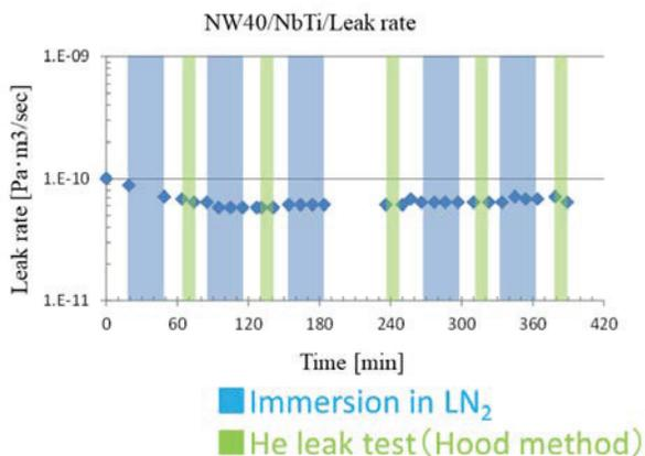
Figure 6: Result of helium leak rate (NW40).
