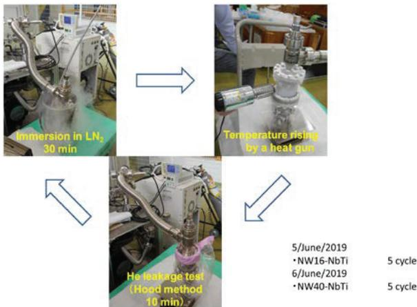
Figure 4: Procedure of the heat cycle test.
