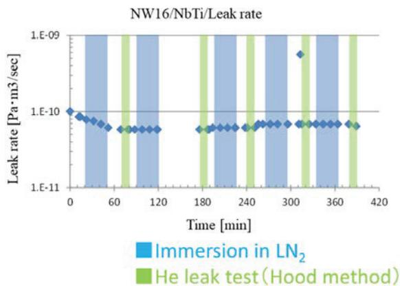
Figure 5: Result of helium leak rate (NW16).
