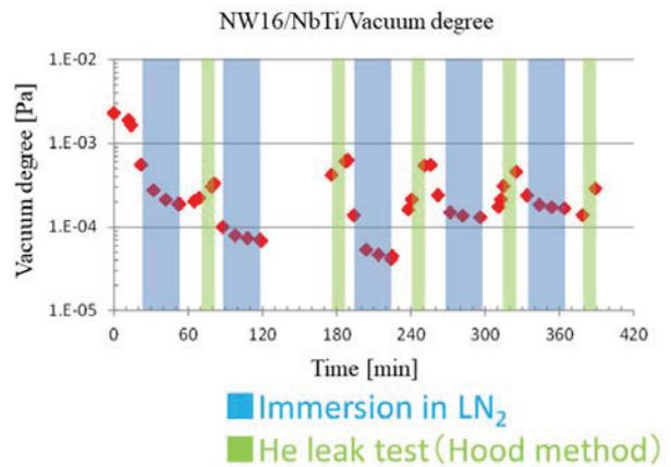
Figure 7: Result of Vacuum degree (NW16).
