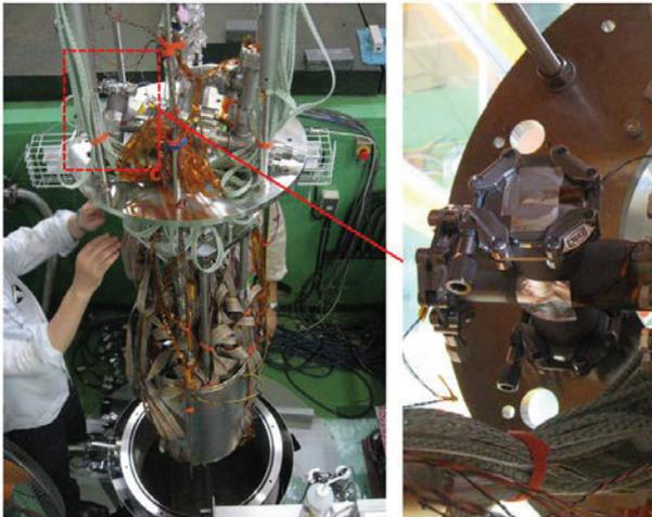
Figure 11: Test flanges installed into the helium vessel.
