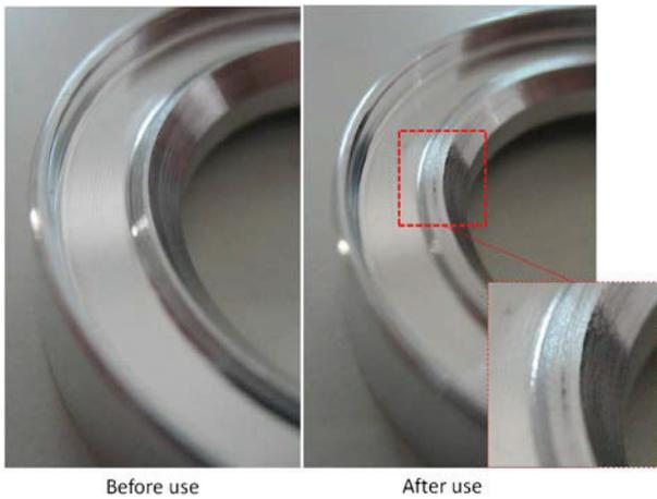
Figure 10: Aluminium edge seal (Before and after use).
