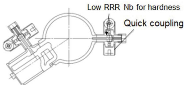
Figure 1: Future plan of the pick-up port with the quick coupling seal.
