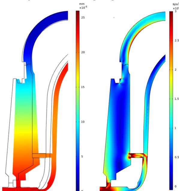
Figure 2: FEM analysis (strain on the right, VM stress on the left) of the spool transition ring while withstanding the reaction force of 10 MV/m cavity field. Peak values in the colour code are 0.25  $\mu\text{m}$  and 0.03 MPa, respectively.
