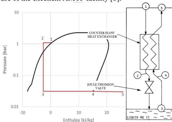
Figure 7: Conceptual layout of the 2 K refilling system for the LASA facility and corresponding points in the pressure-enthalpy graph of helium [9].
