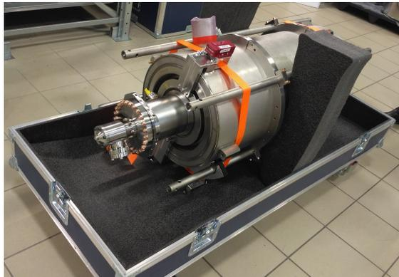
Figure 4: M001 cavity prepared for leaving Zanon. A shock logger (purple box) is visible on the top of the He-tank, above the orange security strap.
