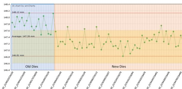
Figure 10: Example of scatter of measurements on length of Inner Dumb Bell before trimming. This is a typical plot available on the ESS Dashboard.
