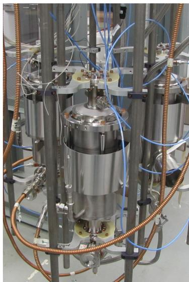
Figure 5: Three 3.9 GHz cavities assembled to the insert, ready for testing in VTS.
