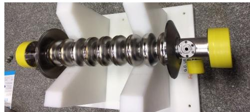
Figure 1: Bare cavity during incoming inspection at Fermilab.
