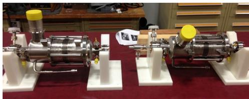
Figure 3: Two dressed cavities during incoming inspection at Fermilab.
