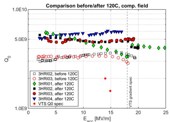
Figure 2: Q vs E performance in VTS for the four design verification cavities before and after 120C bake.
