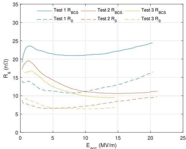
Figure 3: RF test results of the three infusion tests of cavity SC-06.  $R_{\text{BCS}}$  taken at 2 K. Peak field shown here does not indicate quench field.
