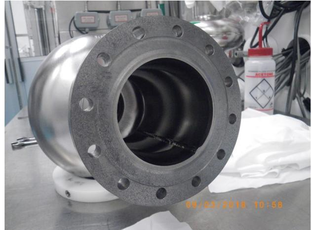
Figure 1: Close-up photo of RDTTD-4 NbTi flange, showing black speckling after initial infusion treatment.
