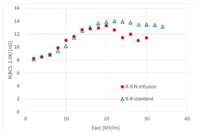
Figure 6: Comparison of deconvoluted BCS resistance at 2.0 K of R-8 cavity for 6<sup>th</sup> N-infusion and reference.
