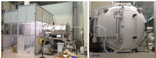
Figure 1: KEK new vacuum furnace.
