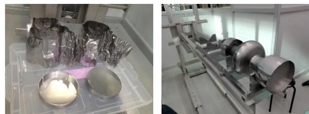
Figure 3: (left) Nb caps and foils to cover flanges. (right) Cavity covered with Nb cap.
