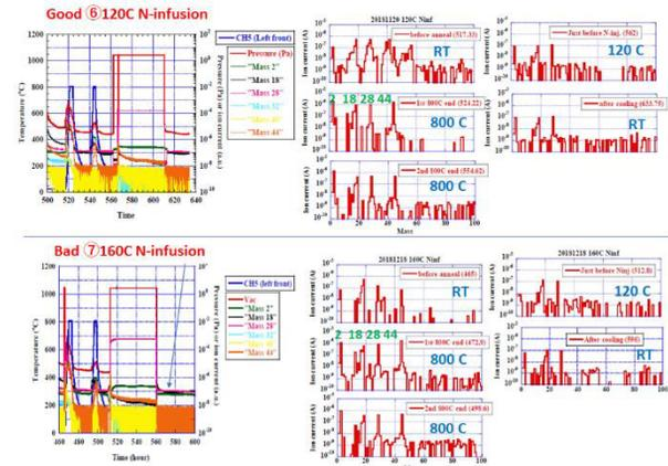
Figure 8: RGA spectrum for good (6<sup>th</sup>) and bad (7<sup>th</sup>) N-infusion runs.
