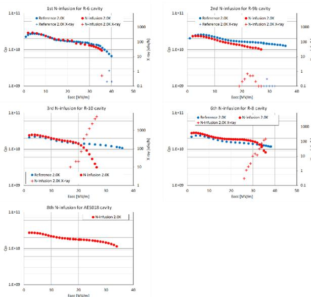
Figure 5: Comparison of vertical test results between N-infusion (red) and reference (blue) for (left-top) 1<sup>st</sup>, (right-top) 2<sup>nd</sup>, (left-centre) 3<sup>rd</sup>, (right-centre) 6<sup>th</sup> and (bottom-left) 8<sup>th</sup> N-infusion. No reference data for 8<sup>th</sup> N-infusion.
