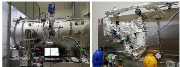
Figure 2: (left) TMP and RGA monitoring system. (right) N-injection system with mass-flow controller.
