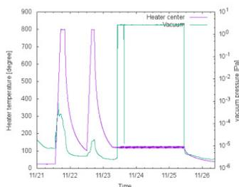
Figure 4: (left) Temperature and vacuum history of typical N-infusion process, which was applied from 6<sup>th</sup> to 8<sup>th</sup> N-infusion runs.
