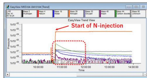
Figure 9: RGA spectrum during Nitrogen injection.
