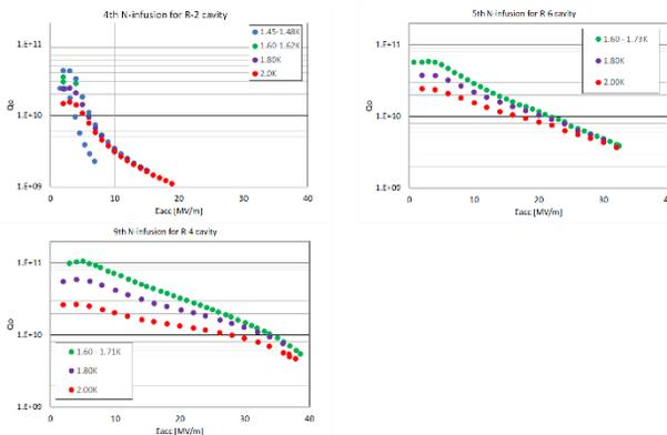
Figure 7: Vertical test results for failed N-infusion: (left-top) 4<sup>th</sup>, (right-top) 5<sup>th</sup> and (left-bottom) 9<sup>th</sup> N-infusion runs.
