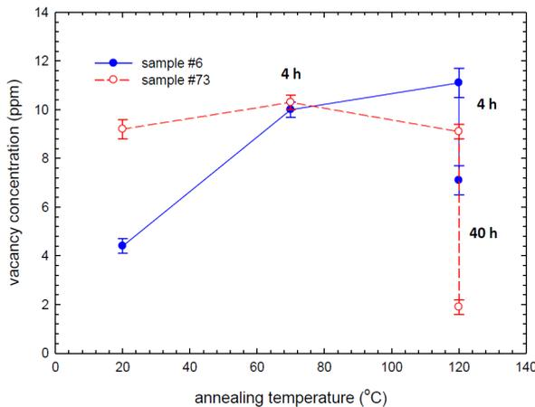
Figure 5: Vacancy Concentration calculated from PALS data using two state positron trapping model vs. annealing temperature at a fixed energy for samples 6 and 73.
