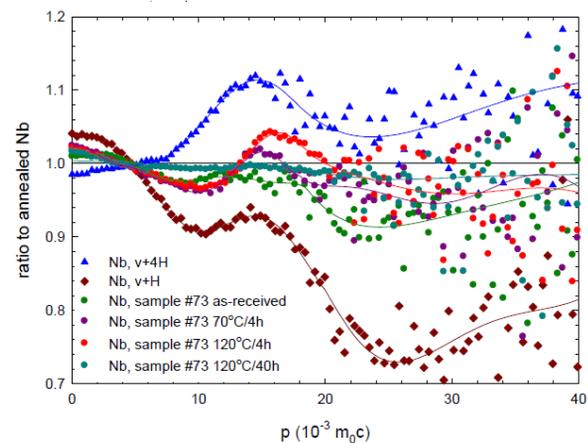
Figure 6: CDB ratio related to pure Nb (annealed at 1000°C) vs. momentum of the annihilating pair for sample 73. Two reference curves for Nb with v+H and v+4H complexes are shown for comparison. While for as-received, some hydrogen is associated to vacancies. v+nH complexes form at 70°C and are stable up to 120°C with short annealing time. After full annealing at 120°C no v+nH complexes are observed.
