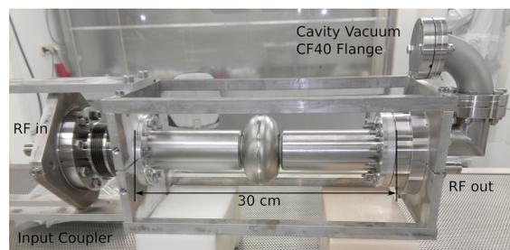
Figure 6: Photograph showing a 3 GHz single cell cavity in the VT assembly. The input coupler is mounted on the left side (top in VT) of the cavity. The as well new designed output coupler is mounted on the right side (bottom in VT) of the cavity.
