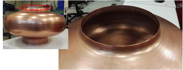
Figure 5: Visual inspection of the defects of the first 400 MHz cavity spun.
