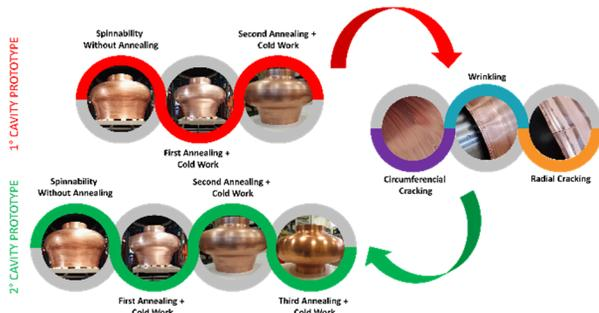
Figure 4: Comparison between the first and the second cavity production steps.
