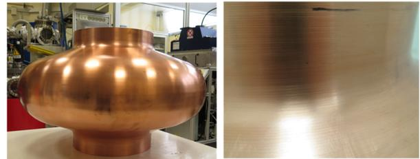
Figure 6: visual inspection of the defects of the second 400 MHz cavity spun.
