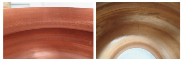
Figure 7: Visual inspection of the surface status of the second 400MHz (on the left the second half cell with an orange peel surface, on the right the first half cell).
