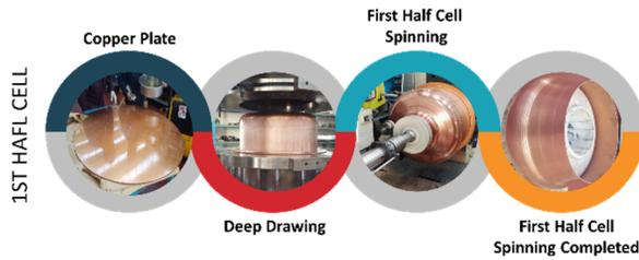
Figure 2: The first half 400 MHz cell spun.
