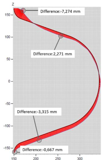
Figure 10: Internal surface profile of the second 400 MHz.
