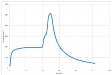
Figure 3: Thermal annealing cycle.
