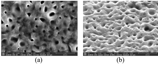
Figure 12: SEM pictures obviously showed many voids on the surfaces of the 2<sup>nd</sup> and 3<sup>rd</sup> batch samples.
