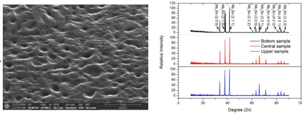
Figure 3: SEM images of the first batch samples tilted at  $55^\circ$  to show three-dimensional features (left); XRD results showed no undesired low- $T_c$  phases were detected (right).
