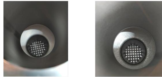
Figure 4: Grey appearance in the downside half-cell; visually non-uniform shiny appearance in the upside cell.
