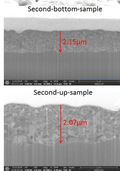
Figure 7: With the modified coating process that kept the Sn source and the cavity at  $1200^\circ C$  for 3 hours, the thickness of the bottom sample and the upper sample is almost the same.
