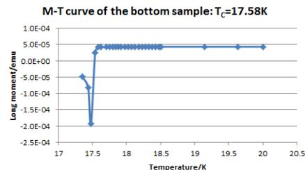
Figure 11:  $T_c$  of the  $Nb_3Sn$  samples coated with the 2<sup>nd</sup> and 3<sup>rd</sup> cavity is about 17.6K.
