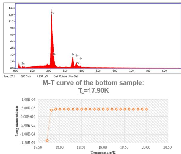
Figure 2: EDS spectrum of the first batch Nb<sub>3</sub>Sn samples indicates composition 24.49 At. % Sn (top); T<sub>c</sub> of the first batch Nb<sub>3</sub>Sn samples reached ~17.9K
